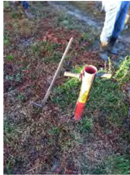
Some tools were at times used to make the plantation easier. This is one of them. Insert the seedling in the pipe and action the pump to plant.
