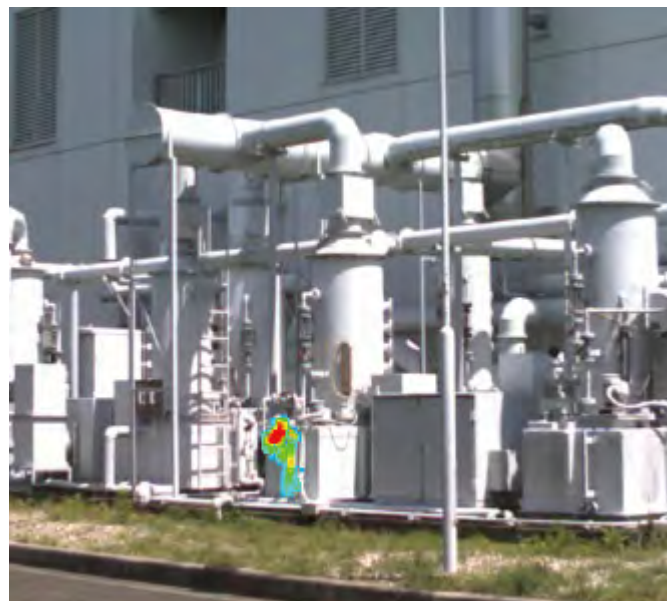
Gas monitoring solution makes gas leaks visible
